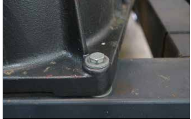
3 - A washer was inserted between the lathe and the stand to fill the gap, before tightening the mounting bolt.
