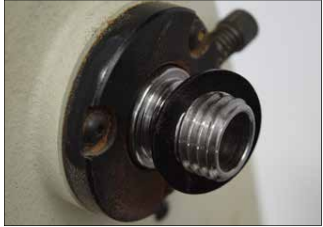
9 - A flat spindle washer can fill a gap between chuck or faceplate and headstock, to improve seating and reduce wobble.
