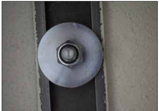
5 - Movable headstocks must be securely locked to the ways. Check the locking plate beneath the ways.
