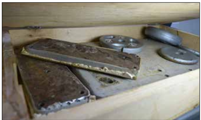
2 - Additional weight helps a lathe absorb vibration. Use steel plate, barbell sets, or sandbags.
