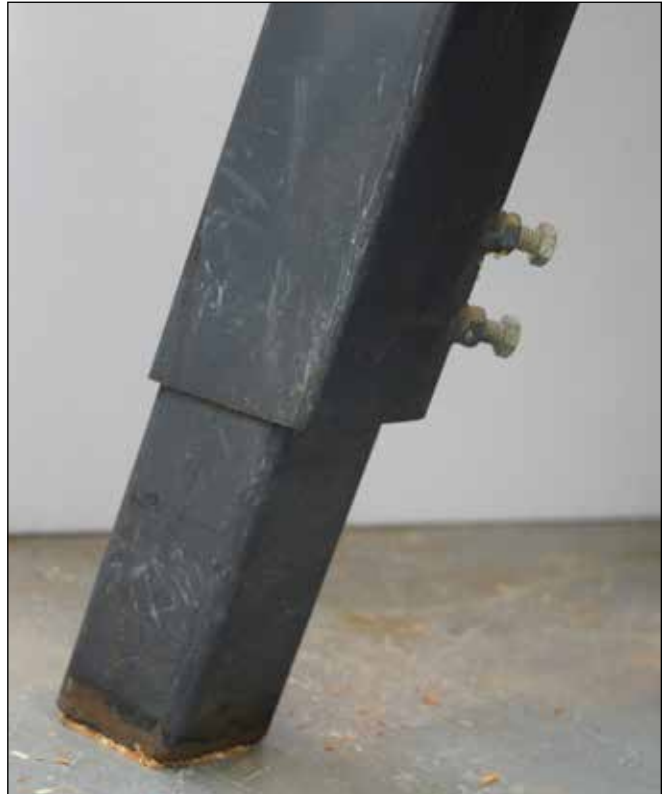
1 - Adjust legs, or use shims, to make sure your stand sits solidly on the floor.
