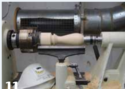
11 The equipment needed for proper sanding goes beyond a stack of abrasives. Personal protection, including a dust mask and dust extractor, is critical.
