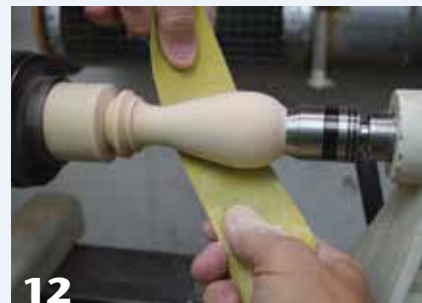
12 Present the abrasive sheet at an angle to efficiently blend curves and remove tool marks. Proceed through the graduated grits, taking care to preserve any crisp details in the form.
