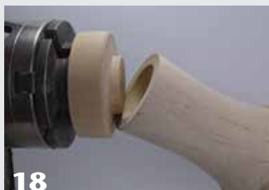
18 A wasteblock held in a scroll chuck is profiled to match the opening of this vase. The tailstock pushes on the form for added security. With the right friction-fit for smaller forms, it is possible to remove the tailstock for final passes on the base.
