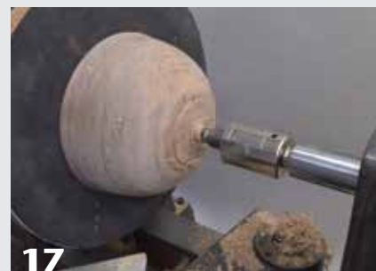
17 A bowl is reverse-mounted by pushing it against the jam chuck with tailstock pressure.
