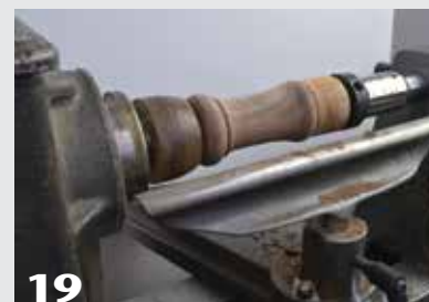
19 Two threaded jam chucks hold this pepper mill blank for turning. One block is threaded on the headstock and a second threaded into a live center adapter. This is one method of driving a form with a through-hole, such as this pepper mill blank.
