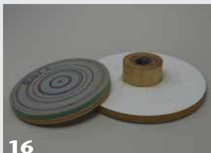
16 Shopmade jam chucks. One (left) is mounted by means of a faceplate and the other with a nut epoxied in a block at the back of the disk. Both are covered with closed cell foam.
