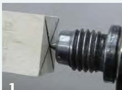
1 Use the tailstock with a revolving center to support the wood until the lighthouse is fully turned.
