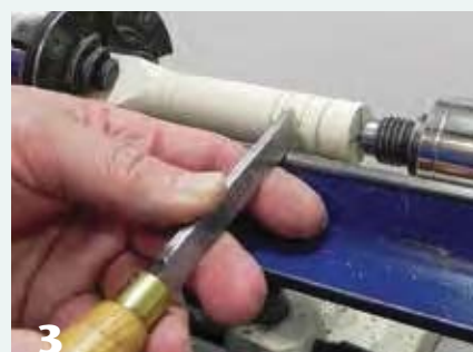
3 Scribe boundaries into the wood using a small skew chisel.
