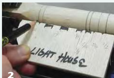
2 Mark key dimensions using a story stick and pencil.
